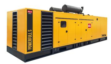
MAIN DATA Continuous power (PRP) kVA 1505.00 Continuous power (PRP) kW 1204.00 kVA Stand-by power (LTP) 1656.00 Stand-by power (LTP) 1324.80 kW 400 - 50 - 0.8 VAC - HZ - cos(fi) Sound pressure 7 m. dBA 74
