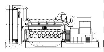
MAIN DATA Continuous power (PRP) kVA 2200.00 Continuous power (PRP) kW 1760.00 kVA Stand-by power (LTP) 2360.00 Stand-by power (LTP) 1888.00 kW 400 - 50 - 0.8 VAC - HZ - cos(fi)
