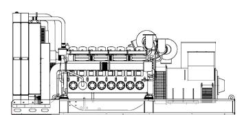
MAIN DATAContinuous power (PRP)1350.00kVAContinuous power (PRP)1080.00kWStand-by power (LTP)1455.00kVAStand-by power (LTP)1164.00kWVAC - HZ - cos(fi)380 - 60 - 0.8KW
