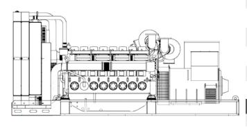
MAIN DATAContinuous power (PRP)1030.00kVAContinuous power (PRP)824.00kWStand-by power (LTP)1110.00kVAStand-by power (LTP)888.00kWVAC - HZ - cos(fi)400 - 50 - 0.8
