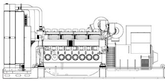
MAIN DATA Continuous power (PRP) kVA 1000.00 Continuous power (PRP) kW 800.00 kVA Stand-by power (LTP) 1100.00 Stand-by power (LTP) 880.00 kW 380 - 50 - 0.8 VAC - HZ - cos(fi)
