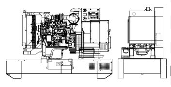
MAIN DATAContinuous power (PRP)100.00kVAContinuous power (PRP)80.00kWStand-by power (LTP)110.00kVAStand-by power (LTP)88.00kWVAC - HZ - cos(fi)380 - 50 - 0.8
