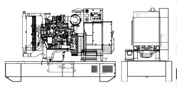
MAIN DATAContinuous power (PRP)60.00kVAContinuous power (PRP)48.00kWStand-by power (LTP)63.00kVAStand-by power (LTP)50.40kWVAC - HZ - cos(fi)415 - 50 - 0.8
