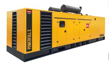
MAIN DATAContinuous power (PRP)1205.00kVAContinuous power (PRP)964.00kWStand-by power (LTP)1290.00kVAStand-by power (LTP)1032.00kWVAC - HZ - cos(fi)380 - 50 - 0.8Sound pressure 7 m.73
