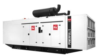
MAIN DATA Continuous power (PRP) kVA 1420.00 Continuous power (PRP) 1136.00 kW Emergency power (E.P.) kVA 1600.00 Emergency power (E.P.) 1280.00 kW 380 - 60 - 0.8 VAC - HZ - cos(fi) Sound pressure 7 m. dBA 79.0
