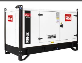
MAIN DATA Continuous power (PRP) kVA 34.90 Continuous power (PRP) kW 27.92 kVA Emergency power (E.P.) 38.20 Emergency power (E.P.) 30.56 kW 380 - 60 - 0.8 VAC - HZ - cos(fi) 69.0 dBA Sound pressure 7 m.
