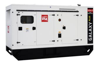
MAIN DATAContinuous power (PRP)225.00kVAContinuous power (PRP)180.00kWEmergency power (E.P.)250.00kVAEmergency power (E.P.)200.00kWVAC - HZ - cos(fi)460 - 60 - 0.8KWSound pressure 7 m.74.0dBA
