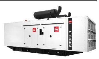
MAIN DATA Continuous power (PRP) kVA 1420.00 Continuous power (PRP) 1136.00 kW Emergency power (E.P.) kVA 1600.00 Emergency power (E.P.) 1280.00 kW 380 - 60 - 0.8 VAC - HZ - cos(fi) Sound pressure 7 m. dBA 79.0
