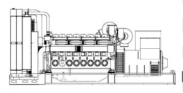
MAIN DATA Continuous power (PRP) 1260.00 kVA Continuous power (PRP) 1008.00 1350.00 kVA Emergency power (E.P.) Emergency power (E.P.) 1080.00 kW 415 - 50 - 0.8 VAC - HZ - cos(fi)
