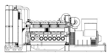
MAIN DATAContinuous power (PRP)1350.00kVAContinuous power (PRP)1080.00kWEmergency power (E.P.)1500.00kVAEmergency power (E.P.)1200.00kWVAC - HZ - cos(fi)380 - 60 - 0.8KW
