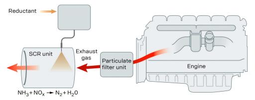
The emissions of particulate matter are filtered through a ceramic structure, that only allows particles smaller than a defined size to pass. When the filter is filled with soot particles to a specific amount, it is regenerated automatically.
