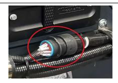
2. Identify the jumper between pin J and D
