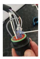
Identify wire 17 connected to pin G of connector X2. Cut wire 17 approximately 10 cm away from the connector, and connect the two wire 17 terminals together with the previously cut wire connected to pin J
